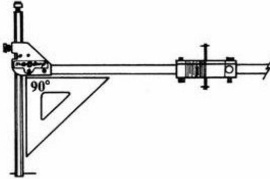
To clean gauges, wipe them off with a rag and cleaning solvent. Should there be an excessive build-up of dirt and grease on the crossbars, fine grit sandpaper and solvent may be used to clean the instrument.
