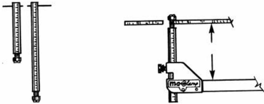
The adjustable scale may be read in either of two ways. The reading may be from the top of the scale holder or it may be from the top of the crossbar. This difference must be accounted for in all cases. A reading of 5" on the scale holder will give an overall reading of 7".
