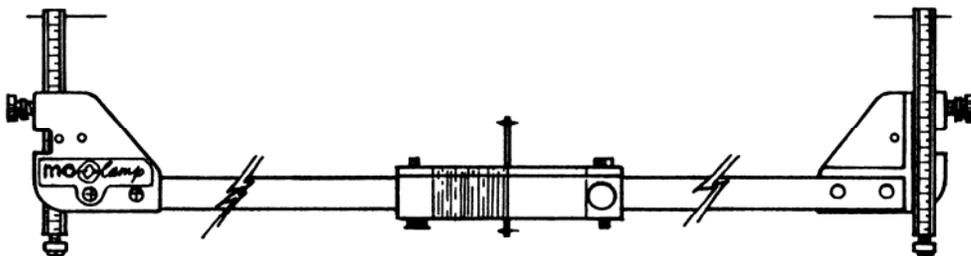
The design of this gauge gives it great durability. However, it must be kept clean and occasionally calibrated. For accurate measurements, the scale holder must remain square with the crossbars.
