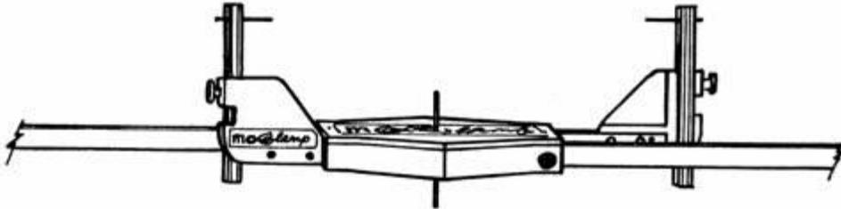
Locking thumb screws are provided in the center of the unit. Locking these screws will prevent the gauge from changing width and falling from the vehicle during the repair procedure. If it is necessary for the gauge to flex in width during the repair of the vehicle, the locking screw should be loosened.
