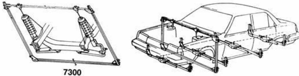
After attaching the strut tower gauge to the vehicle, and adjusting the vertical scales to the proper height, the center sighting pin on the lower horizontal bar should visually line up with the centerline gauge sighting pins if the upper body dimensions of the vehicle are correct. Additional measurements may be taken with either a tape measure or a tram gauge to assure that other dimensions from the datum line and/or centerline are correct.
