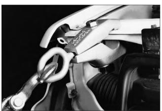
Self-tightening. Great for single-lip flanges and inside frame horns. Original wedge, cross-hatch tooth design, spring-loaded for easy opening. Throat clearance of 1 1/2'' high (38 mm), 1 1/4'' deep (32 mm).
