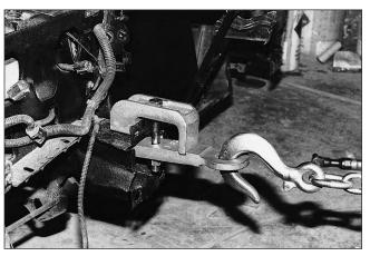
A must for pulling on box rails with welded-on bumper flanges. Large opening to reach around flanges and other obstructions. Its heat-treated jaws grip a substantial area for pulls from several directions and angles. Gator tooth design.
