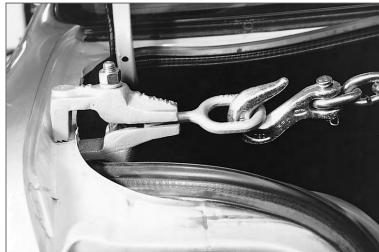
The #0655 Dyna-Mo<sup>™</sup> Box Clamp's heat-treated jaws reach around flanges and other obstructions to get a grip on hard-to-reach surfaces.
